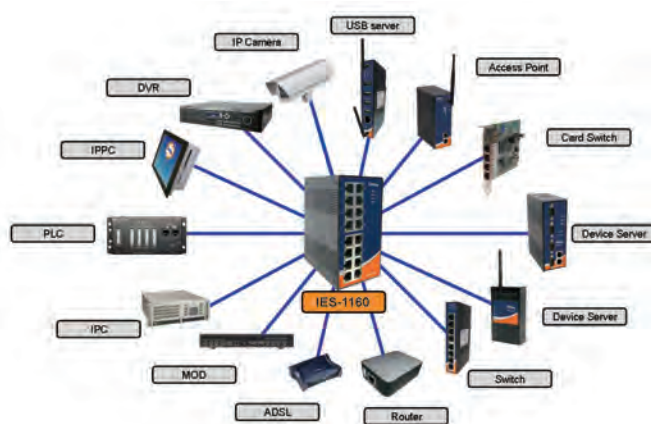
Connections of Ethernet devices
